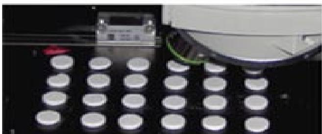
**Figure 3.** 24 tablet plate for the **RAMAN WORKSTATION™** Raman analyzer.
