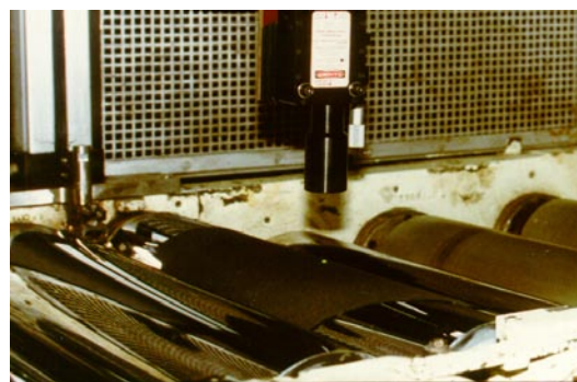
Figure 4. Monitoring a moving polymer film line.
