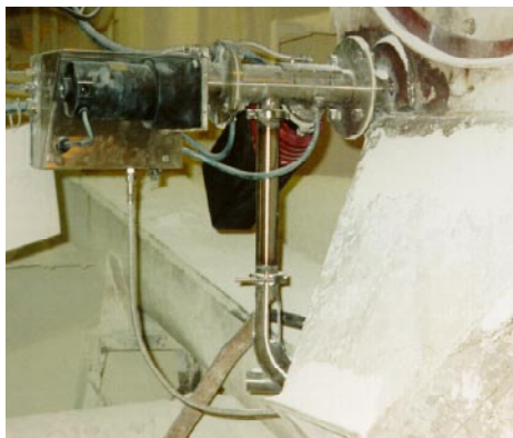
Figure 4. The Raman sampling interface in place on a TiO 2 process line.
