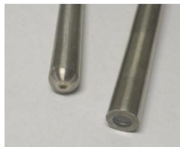
**Figure 5.** View of the tip of an IO. Standard Kaiser shaped tip (left) and traditional flat tip (right).
