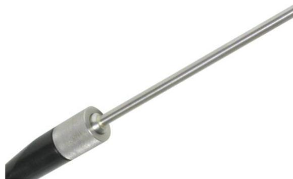
**Figure 4.** View of the cap of the MR Probe probe head that is used to secure the immersion optic.
